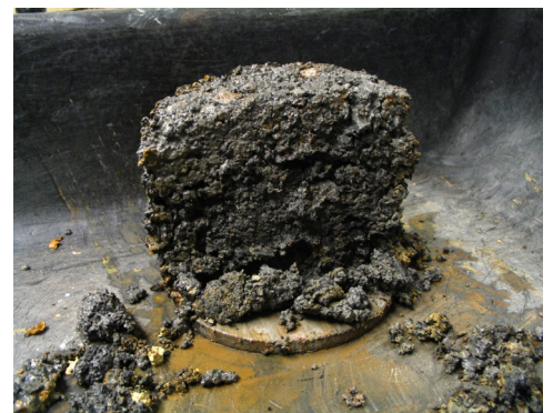
Portion of pyritic shale sample following laboratory free swell test.
